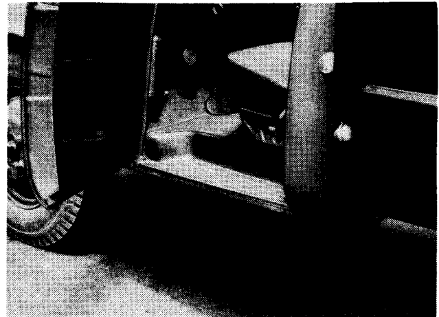
VIEW OF AUXILIARY STEP AFTER INSTALLATION AS OUTLINED ABOVE AND IN DRAWING AT RIGHT
