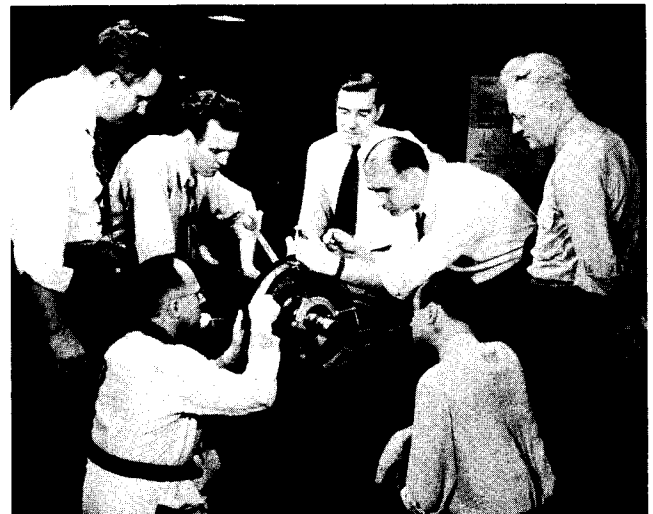
BRAKE ADJUSTMENT made easy. In this picture, students are learning to use a brake adjusting tool.
