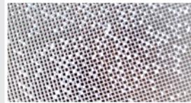
LEFT: Section of DPF showing channels blocked by lube-ash deposits from high-ash oil (white areas.)
