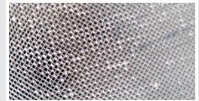
RIGHT: Similar section from engine using ~1% ash oil, such as Shell ROTELLA® T Triple Protection® showing less blockage (fewer white areas.)
