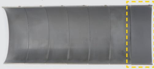
\* New Bearing shown for comparison. Note very little evidence of wear or corrosion on the left side after almost 600k miles.
