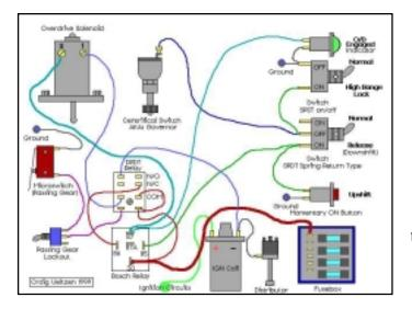
This is a diagram for wiring a split shift control setup for your T-85N transmission. This can be used for one you've bought outright and have no original circuits for, or modifying the one you already have. The DPDT relay is a **D**ouble **P**ole **D**ouble Throw relay. Radio Shack carries them. The passing gear lockout switch is for when you want to run flat out without it dropping out of top gear.
