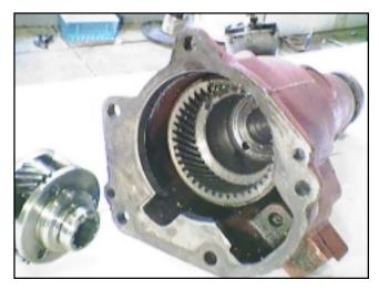
The overdrive solenoid with the cover removed. When powered, the shaft puts pressure on locking dogs until engine torque is released, then the locking dogs engage the planet set case, and the ring gear then rotates 27% faster than the input shaft. The large terminal is the (S)olenoid line, and the (I)gnition terminal has a short to ground when the shaft is in the engaged position.
