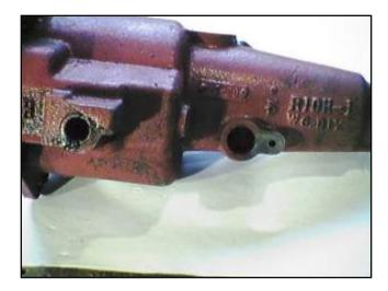
This is a Borg Warner T-85N case with the componants removed. The hole on the left is for the freewheel clutch lockout. The right hole is for the speedometer. These photos are of my spare overdrive unit.
