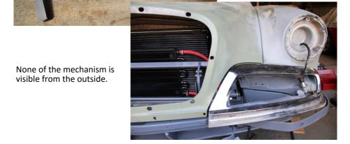
In this picture you can see the catch arm which is part of the mechanism.
