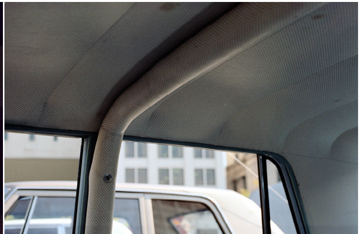
A roll bar was installed on all twenty of the demonstrator units. It is possible a few more were installed on other 1964 Marshals that were not part of this special run of demonstrators.
